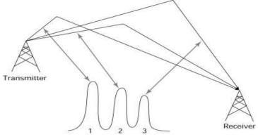
Fig.1 A Multipath Propagation Scenario
