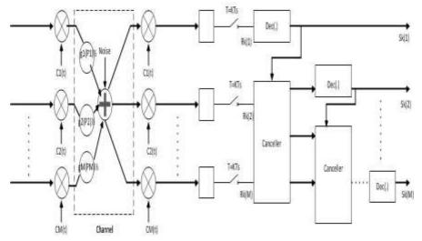
Fig.3 Successive Signal Detection Approach
