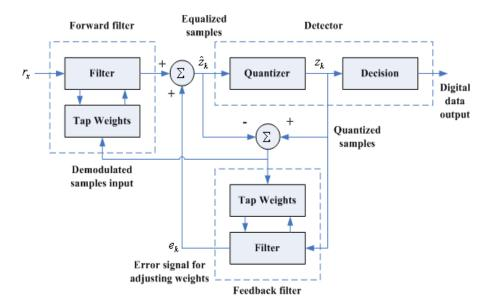
Fig.2 Block Diagram of a Decision Feedback Equalizer (DFE)
